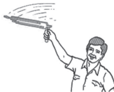
Figure 37-27. Technician spinning a wet-bulb and dry-bulb thermometer, known as a sling psychrometer.
